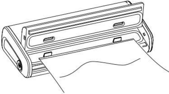
3. Close lid by pressing down on both sides. If you hear a "click" on each side, then you have successfully locked the lid in place.
